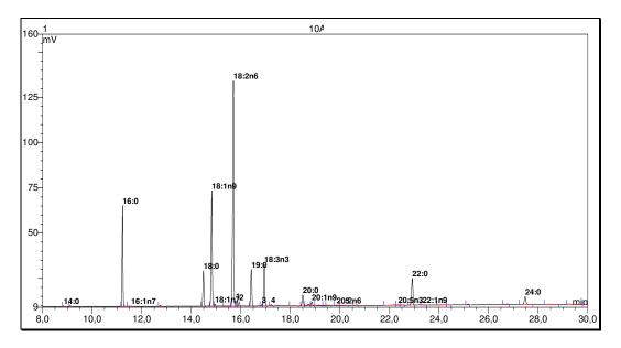
Fig. 1. Chromatogram of fatty acid methylesters from *Tephrosia vogelii* crude oil. GCMS conditions: Agilent 6890N auto sampler 7683B series; Stationary phase: Polyethylene-glycol (PEG); Mass Selective Detection: Ionization energy, 70 eV; source temperature: 230 °C; The injector temperature: 260 °C; Column: CP WAX 52CB 25m X 0.25mm (i.d), thickness of 0.2µm; Standard Mixture (20FAME): GLC-68A from NuCheckPrep Elysian, WO
